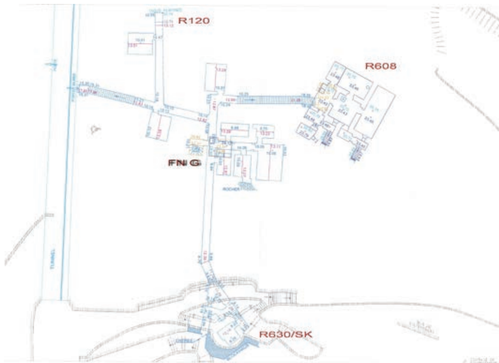
The kaverne tunnels in Biarritz have dozen of rooms excavated in limestone rock
